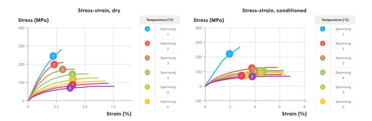
Test run at 23°C if not differently specified, DAM state (dry as moulded). \*: conditioned according to ISO 1110
